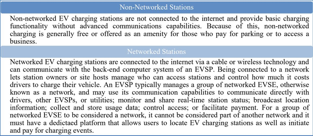
**Figure 1. Non-networked vs. networked EV charging stations**
